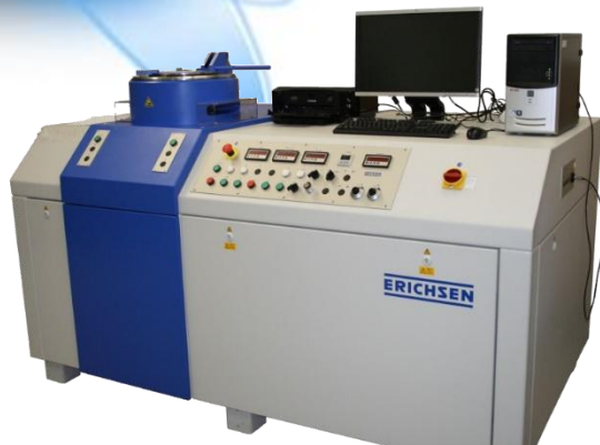
Erichsen 145-60 unique universal testing equipment for technological testing of metal sheets
