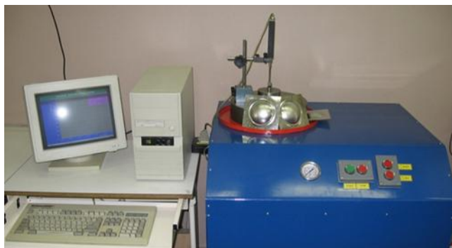
Equipment for Bulge test for US Steel Košice
